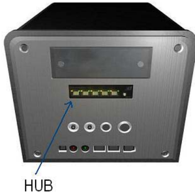
Figure 2.2.1: PhaseSpace server computer with integrated HUB
